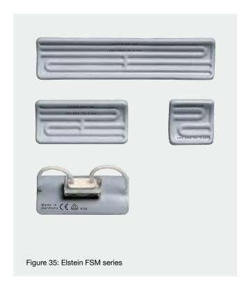
Elstein MaxLife FSM panel heaters are ceramic infrared heaters, which are designed for operating temperatures up to 720 °C. Surface ratings of up to 64 kW/m² can be installed.
