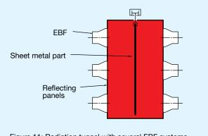
Figure 11: Radiation tunnel with several EBF systems
