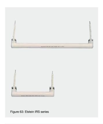
Elstein IRS rod heaters are ceramic infrared heaters, designed for operating temperatures of up to 650 °C. With the help of MPO and MPO/2 mounting profiles, surface ratings of up to 72.0 kW/m² can be realised.
