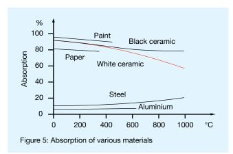
Infrared radiation is the term used to describe the emission and transmission (propagation) of electromagnetic waves within the spectral range above visible light from 0.7  $\mu m$  up to around 80  $\mu m$ . This emission and transmission of the electromagnetic waves is associated with the specific, directional transport of energy. The transmission of energy does not require a transport medium and is therefore also possible in a vacuum.
