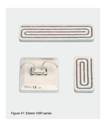
Elstein HSR high speed heaters are quick-reaction ceramic infrared panel heaters, designed for operating temperatures up to 860 °C and surface ratings up to 64 kW/m².
