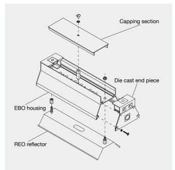
Figure 97: Example for the arrangement of metal parts using an EBO housing with REO reflector
