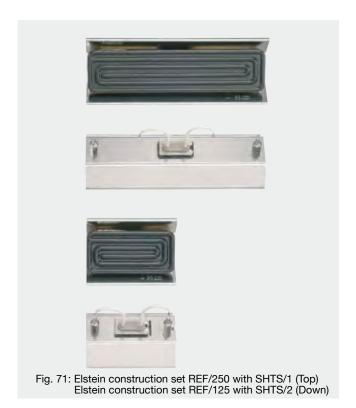
By quoting the REF/250 or REF/125 construction set designations and the heater type required, the REO/250 and REO/125 reflectors are available fitted with the FSR, FSM, HFS, HSR, HTS and SHTS series ceramic infrared panel heaters.
