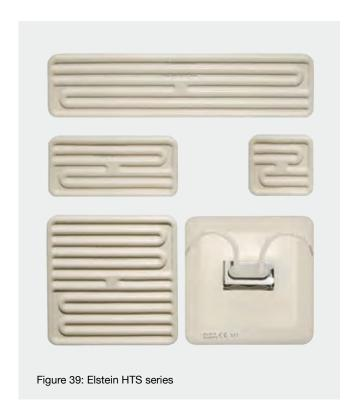
Elstein HTS high temperature heaters are ceramic infrared panel heaters, which can be used for operating temperatures up to 860 °C and surface ratings up to 64 kW/m².
