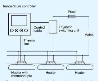
Figure 23: Block diagram of the temperature control circuit
