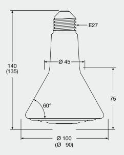
Figure: 68 Mounting dimensions and heater dimensions () in mm
