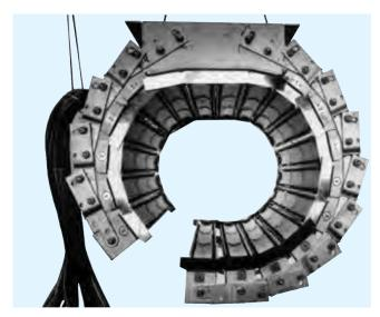
Figure 28: Heating head for heating GRP pipes
